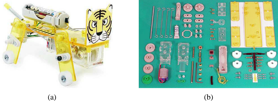
Figure 1: TAMIYA® Robot Kit - Mechanical Tiger: a) assembled and b) parts in the kit 7
